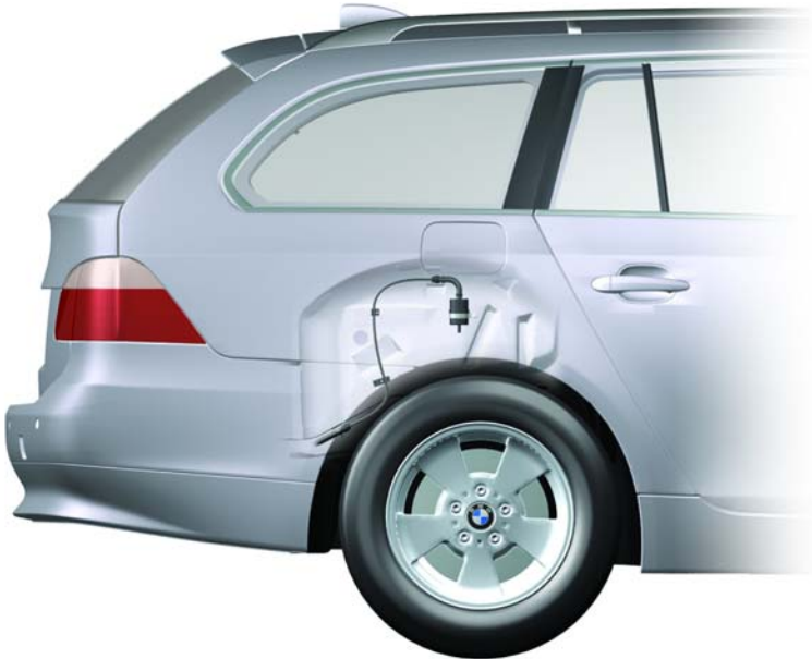
Location of air filter for LVA
